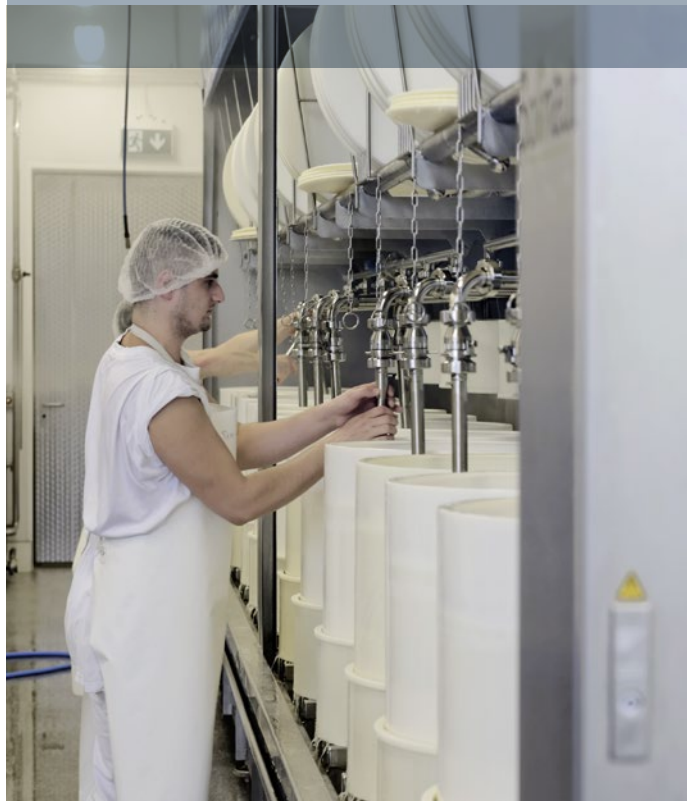
For further processing, the cheese flakes, including the whey, are pumped into large round molds and then pressed
